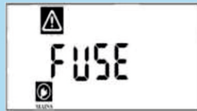
Mains Fuse Blown / MCB Tripped
